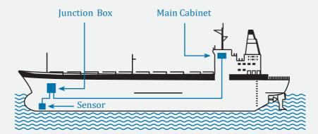
The flat sensor surface measures the water speed along the hull. The sensor must be located near to the bow, as far forward as possible. It must always remain immerged.
