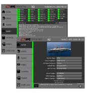
An incident marker control is present on each page to allow the user to add an entry into the event log for ease of data playback, with a "test on demand" feature which tests all aspects of the system as required.
